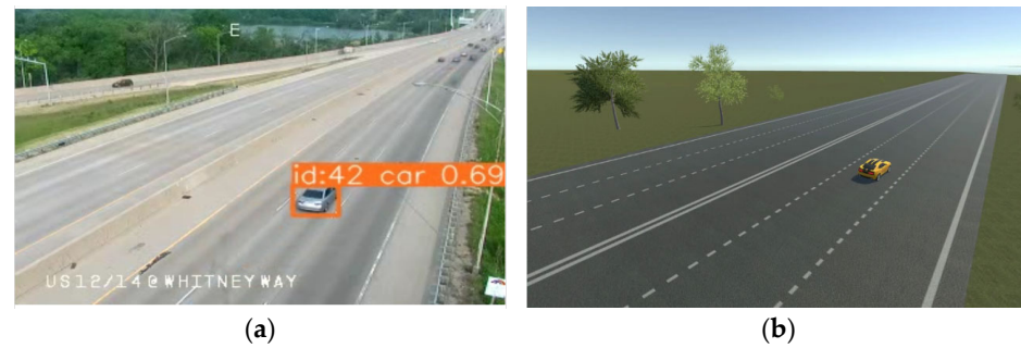
Figure 8. Video recognition and Unity-based DT model. (a) Physics world video. (b) Digital simulation.
